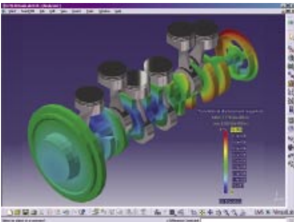
By coupling a flexible model of the crankshaft to the engine block finite element model through sophisticated oil film models, internal loads can be accurately predicted and used for further downstream analysis.
