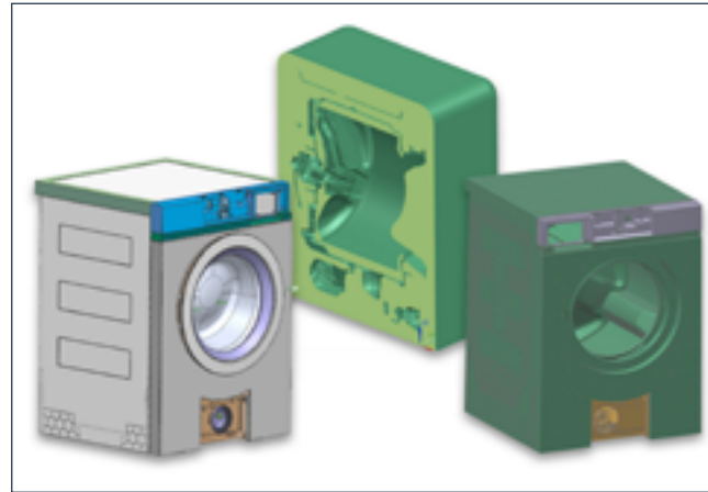
Structural and air model derived from the CAD model and coupled to the vibroacoustic model. (below)
